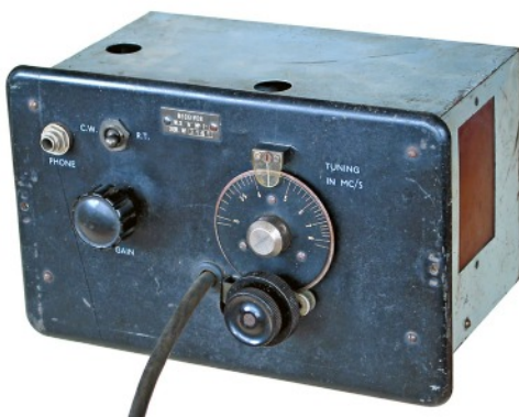
The receiver part of the British SOE A Mk.1 was electrically very similar to that of the Wireless Set No. 1 MARK 1. (See circuit diagram above.)
